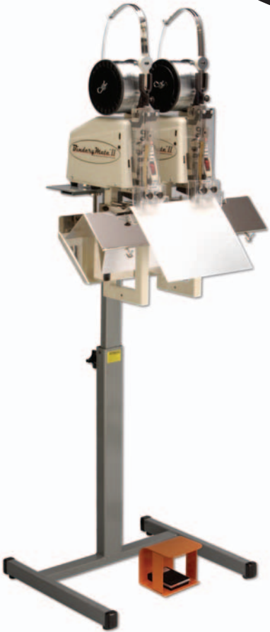
Dual unit shown with optional stand *stand height adjusts from 29" to 41" *stitch centers from 4 1/2" to 12"
